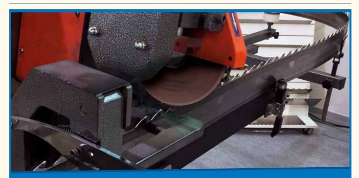
Improved performance of grinding applications of strip and circular saws with a renewed formula. In particular, the secretion / balancing problems of the stones have been completely eliminated. The results of applications in the working areas support the increase of demand of completely new products.
