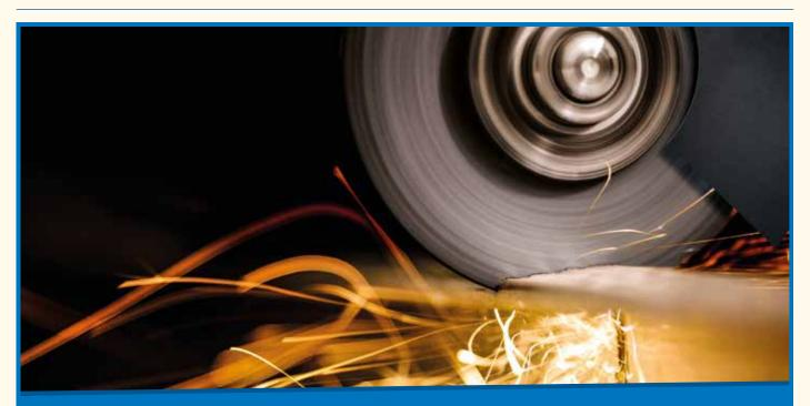
In New Zirconia (ZA) Thin Line Cut-Off Discs, addition of zirconium oxide provides 25% increase in stainless steel cutting performance in particular. Higher performance was also achieved when cutting thin stainless steel sheets. The use of these abrasives, especially in precision casting, will increase productivity.
